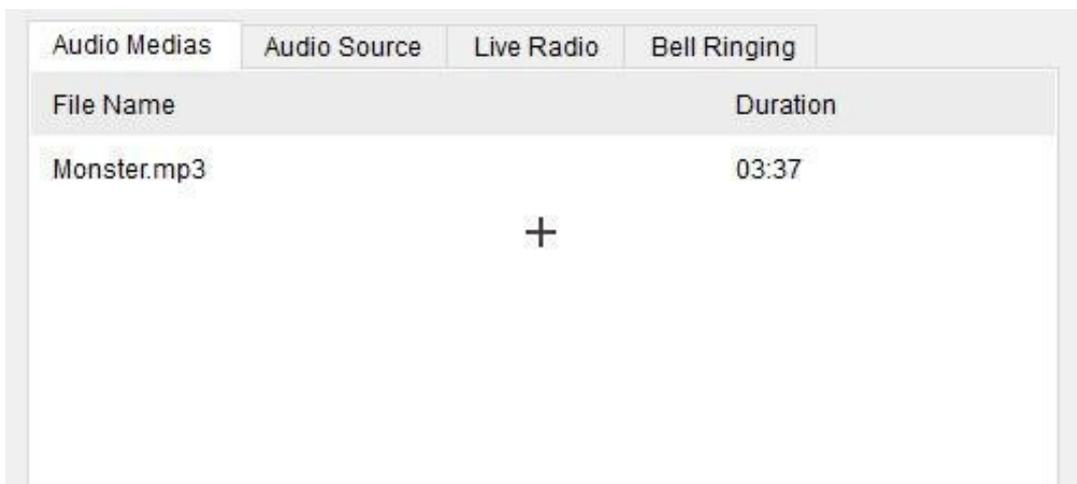
Audio source: There are two ways, one is live microphone in, you can announce directly in PC or a connected microphone. And the other one is the system could detect the signal from outside music player like spotify and then auto playing.
