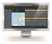
The 2N® Lift8 Communicator is a user application for the administration of alarm calls. In the event of an incoming emergency call, all data about the lift is displayed, including a map with information on the location of the lift and the option of making notes. This is a VoIP client. A condition for operation is the installation of 2N® Lift8 Server software on any computer and connection to the same network as the 2N® Lift8 Communicator.
